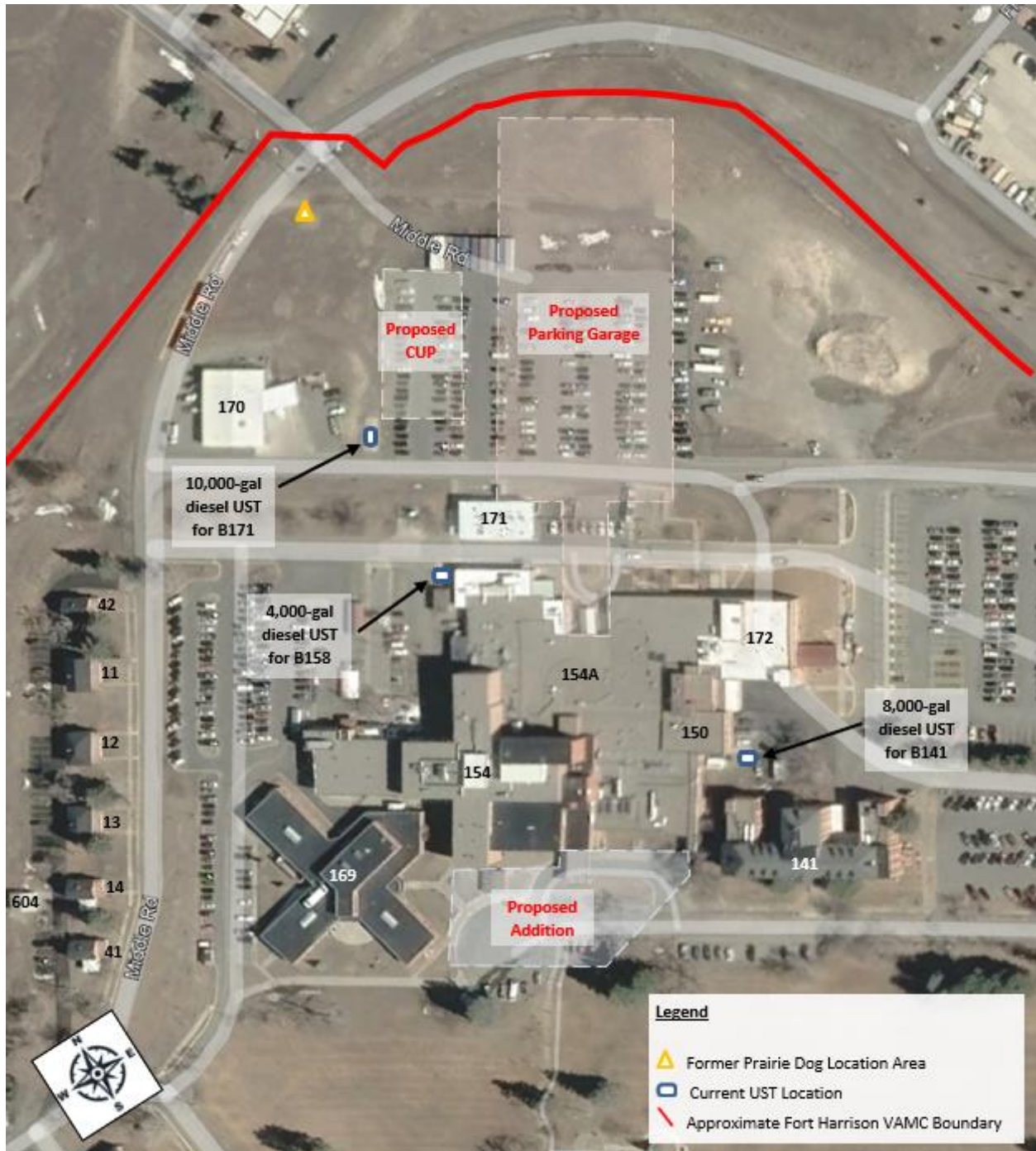
Figure 3-8 Current UST Locations
