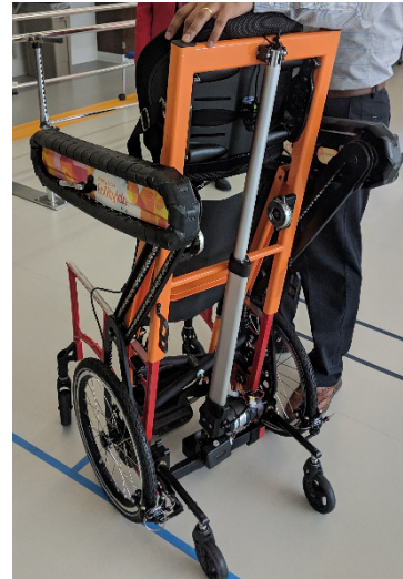
Experimental standing wheelchair built with bicycle engineering.
